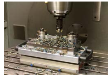
Double clamp fixture with clamping plate
